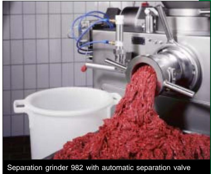
Separation grinder 982 with automatic separation valve
